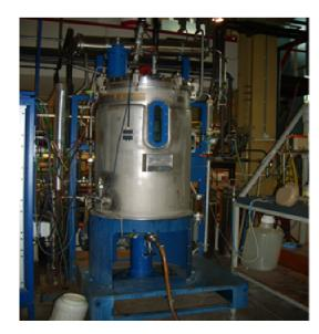
Figure 9. Pilot-scale fed-batch fermentor for the study.
