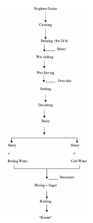
**Figure 1.** Flowchart for the production of kunun drinks by wet milling methods.
