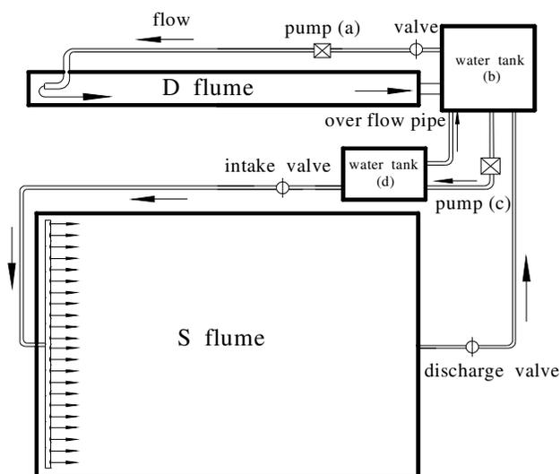
**Figure 1.** Experimental design for hydrodynamic and hydrostatic flumes.
