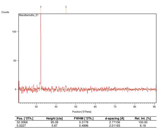
**Figure 2.** The XRD Image of silver nanoparticles synthesised using Sunflower leaf extract. The diffraction patterns were obtained by measurement of angles at which X-ray beam is diffracted by the crystalline phases in the specimen. X-ray diffraction (XRD) measurement of the bio-reduced silver nitrate solution dropcoated on glass substrate bio-film was carried out on a Philips PW 1830 instrument operating at 40 kV and a current of 30 mA with Cu  $K_a$  radiation.
