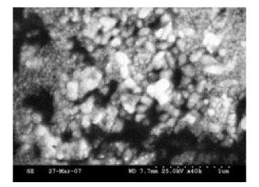
Figure 3. The SEM image (WD 7.7 mm 25.0 kV x 40 k) of silver nanoparticles synthesised using sunflower leaf extract. Dried suspension of silver nanoparticles synthesized by reduction of silver ions in water was subjected to electron microscopy (SEM) using Hitachi made Scanning Electron Microscope of Model No.S3000H at central electro chemical research institute
