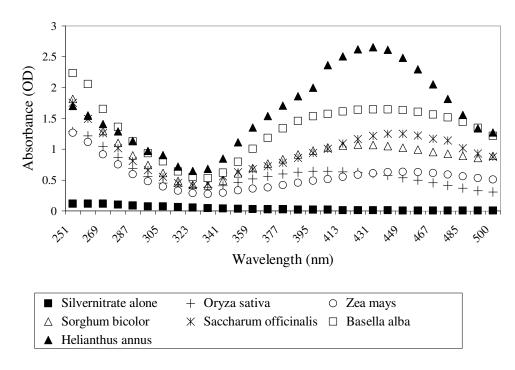
**Figure 1.** UV visible absorption spectra recorded as a function of time of reaction at  $10^{-3}$  M aqueous solution of silver nitrate with different leaf extracts. The silver nanoparticle formation was monitored through UV-Visible absorption spectroscopy (excitation band near 430 nm for silver) at regular intervals as a function of time of reaction on a Genesys 10-UV Thermo Spectrophotometer operated at a resolution of 3 nm.
