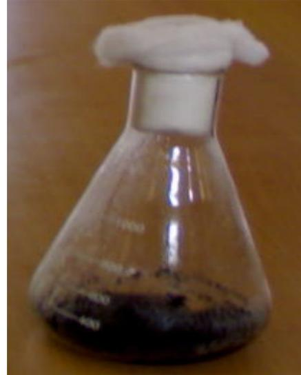
**Figure 3.** Solid state fermentation flask.
