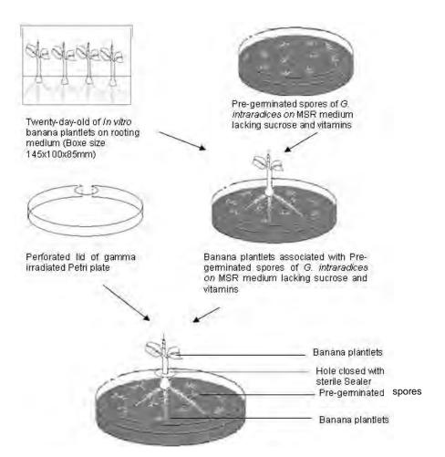
Figure 1. Cultivation system for the in vitro mycorrhization of banana plantlets.
