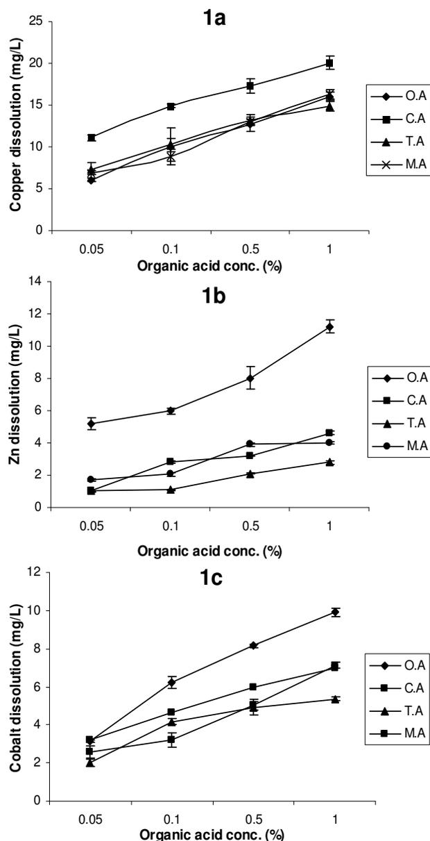
**Figure 1.** A plot of chemical leaching of metals by organic acids after 30<sup>th</sup> day (a) copper (b) zinc (c) cobalt. O.A = oxalic acid, C.A = citric acid, M.A = malic acid and T.A = tartaric acid.
