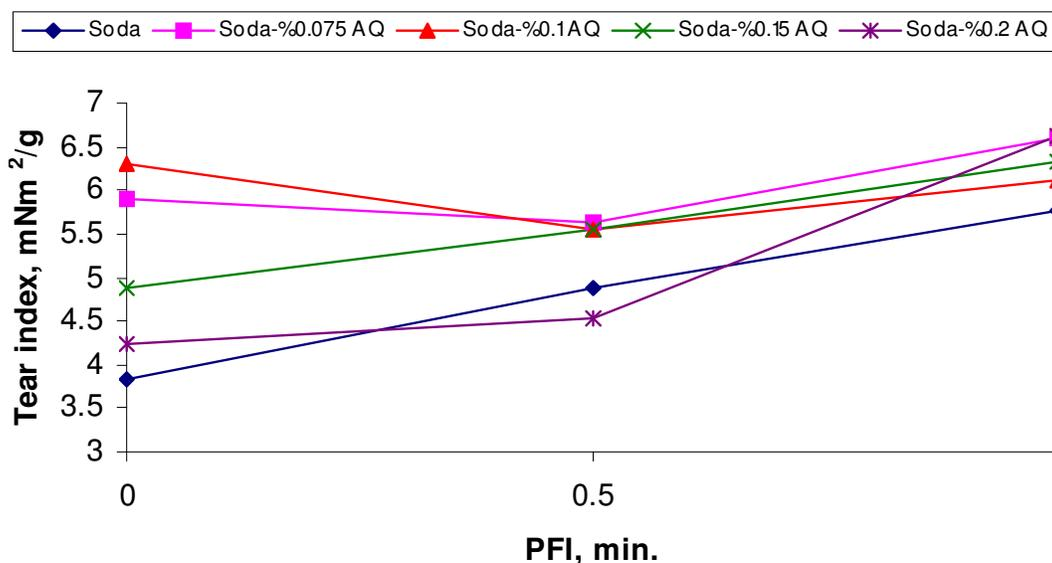
Figure 5. Effect of AQ on tear strength.
