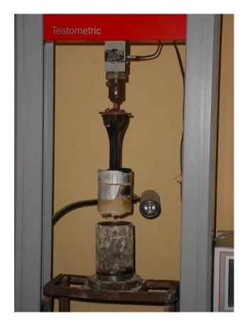
**Plate 1.** The Piston-Cylinder assembly on the Universal Testing Machine.
