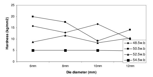
Figure 3. Effect of die diameter on hardness at different moisture content level.
