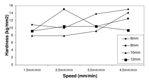
Figure 2. Effect of speed on hardness at different die diameter.
