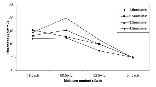
Figure 1. Effect of moisture content on hardness at different speed levels.
