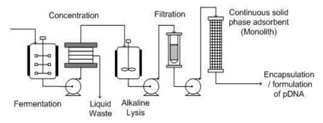
Figure 2. Proposed process flow sheet for single-stage purification of plasmid-based therapeutic products (Danquah et al., 2008b).
