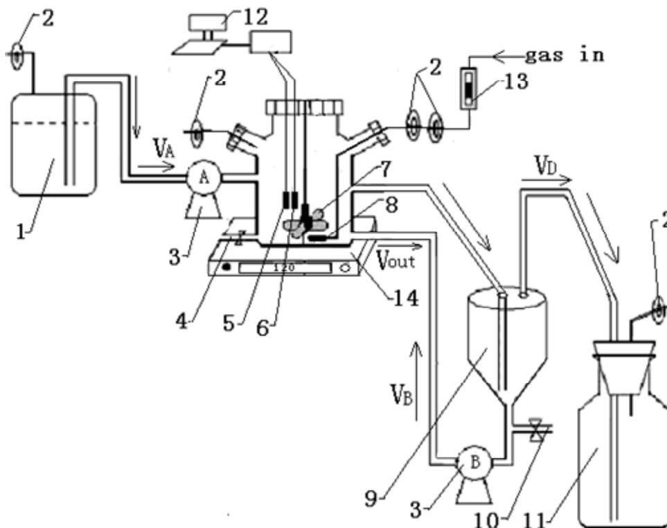
**Figure 1.** Configuration of perfusion stir-tank bioreactor system. 1) Fresh medium; 2) Air filter; 3) Pump; 4) Sample pipe; 5) pH probe; 6) DO probe; 7) Impeller; 8) Air sparger; 9) Settlement device; 10) Cell harvest pipe; 11) Discarded medium; 12) Computer; 13) Air flow meter; 14) Magnetic churn-dasher.
