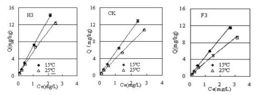
**Figure 3.** Sorption isotherms for imidacloprid on soils (n = 3). H3 and F3 refer to exogenous HA and FA added to soil to enhance the amount of soil organic carbon (SOC) by 10.0 g kg<sup>-1</sup>, respectively.
