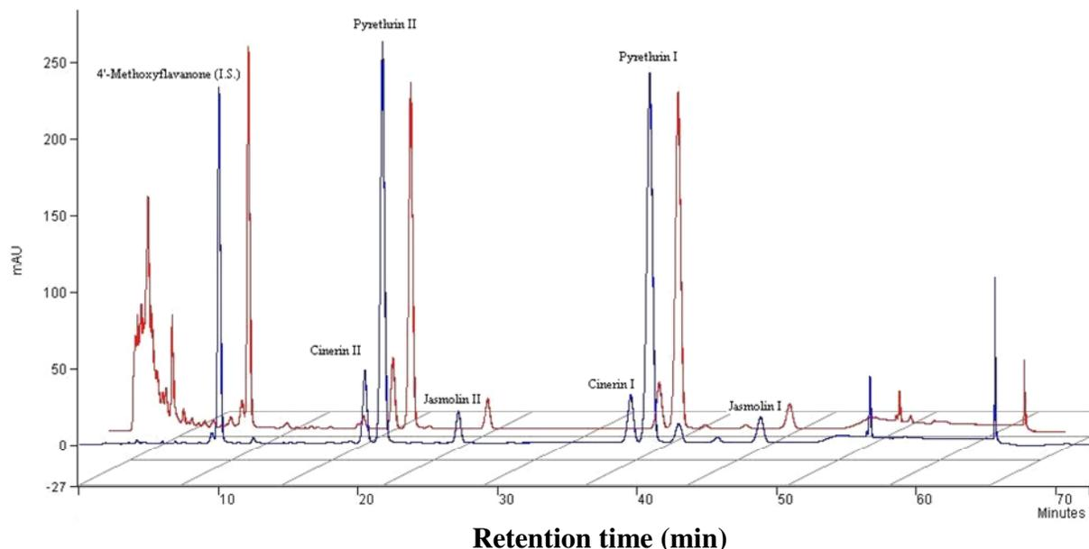
**Figure 2.** Reversed-phase HPLC chromatogram of standard (blue line) and sample (red line) of pyrethrum extract. (Mobile phase flow rate  $1 \text{ mL min}^{-1}$ , injection volume  $20 \mu\text{L}$ , UV detector at  $230 \text{ nm}$ )
