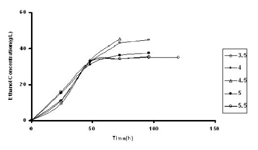
Figure 2. Effect of pH on ethanol production.
