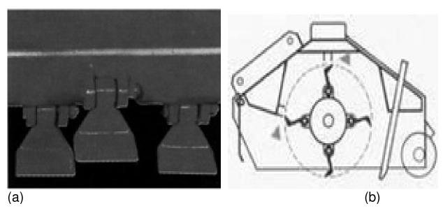
Figure 2. Hammer-type blades of the splined-type stalk chopper.
