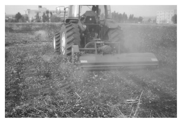
Figure 1. Splined-type stalk chopper.
