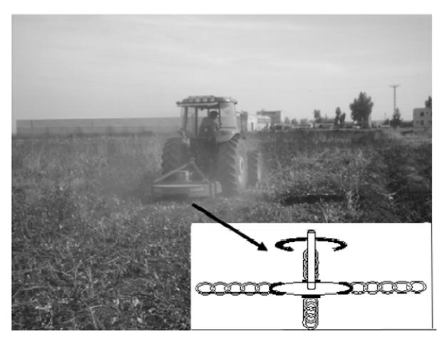
Figure 3. Chained-type stalk chopper.
