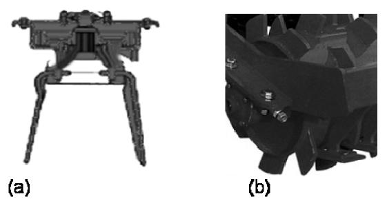
Figure 5. Blades and cylinder gears of vertical-blade rotating dredge
