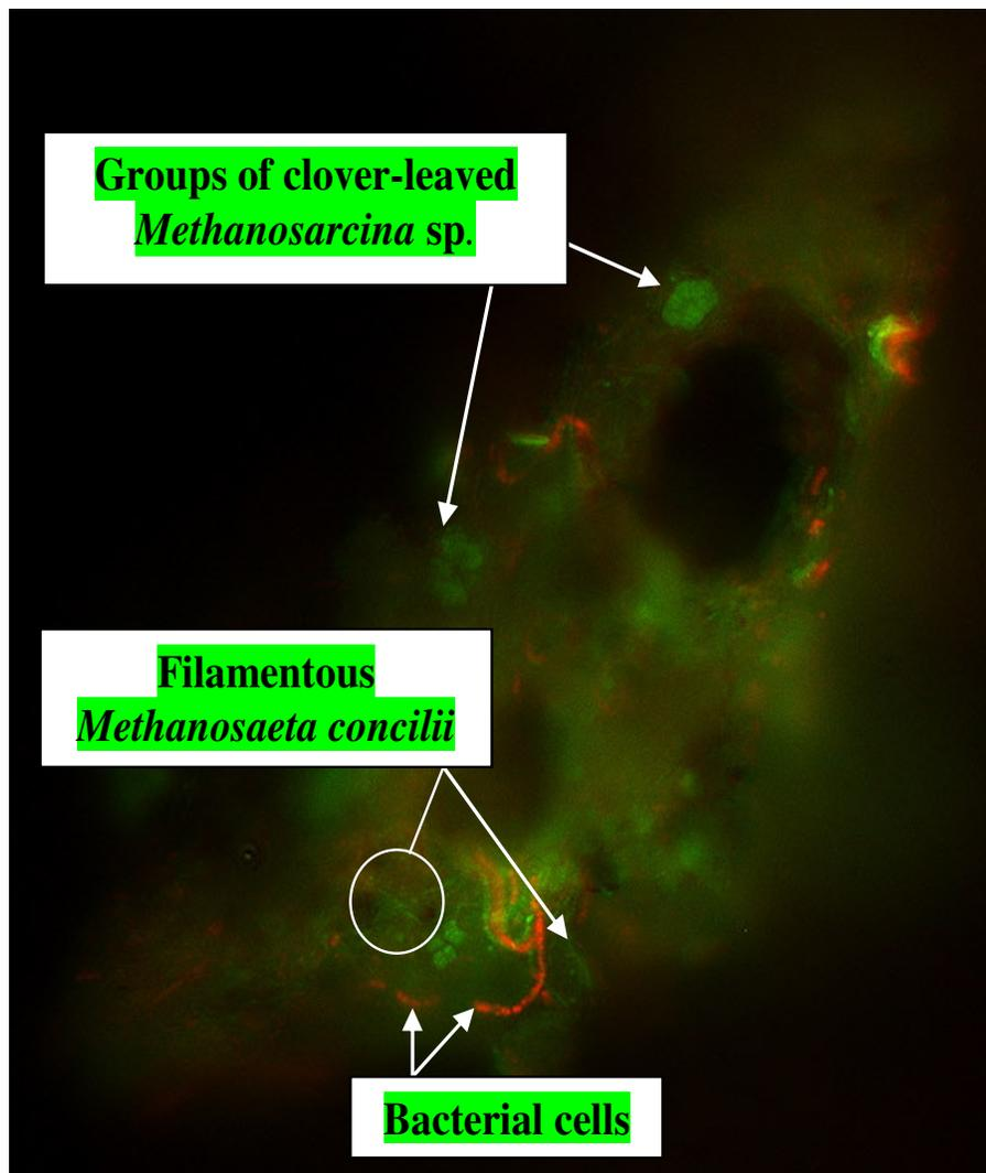
**Figure 7.** FISH staining of the sludge samples analyzed by confocal laser microscopy of fluorescent *in situ*-hybridized cells. A flocs simultaneously hybridized with rhodamine-labeled bacterial-domain probe (EUB338, EUB338-II and EUB338-III) (red) and FITC-labeled methanogens probe (MSMX860) (green) showing the distribution of the only two methanogens (*Methanosarcina* sp. and *M. concilii*) and bacterial cells at 400X magnification.
