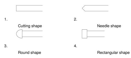
Figure 2. Type of electrodes use in ozonizer; 1) cutting shape, 2) needle shape, 3) round shape, and 4) rectangular shape.
