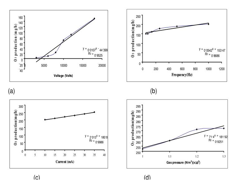
**Figure 3.** Influence of selected factors on ozone production; a) voltage (volt), b) current frequency (Hz), c) electrical current (mA), d) gas pressure (N  $m^{-2}$ ), and e) electrode distance (m).
