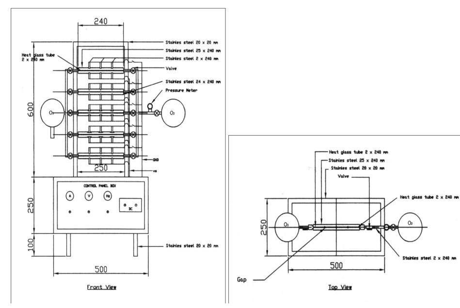
Figure 1. Schematic diagram of a pilot scale ozonizer.
