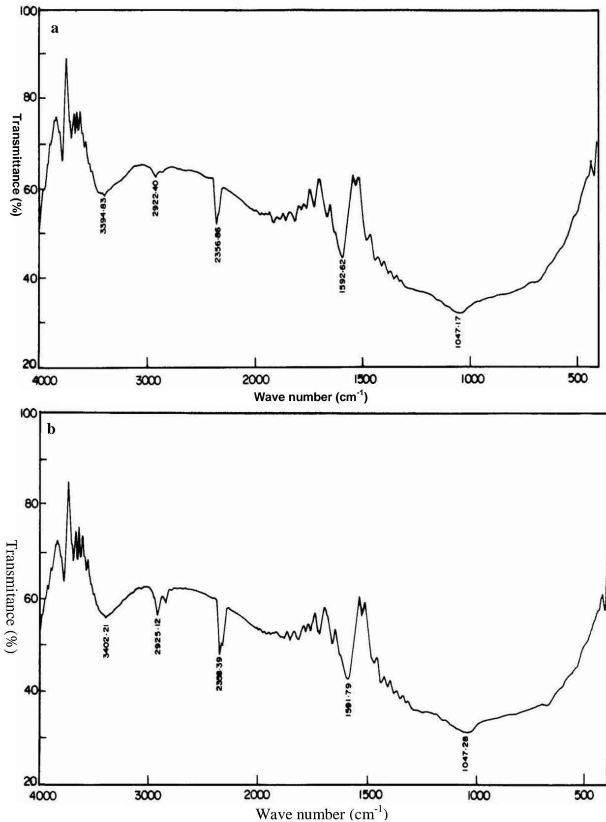
**Figure 4.** IR spectrum of standard taxol (a) and fungal taxol (b) showing finger print region between 1000 and 4000  $\text{cm}^{-1}$ .
