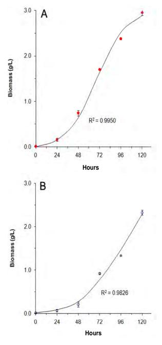
**Figure 5.** Biomass kinetics of *Aspergillus niger* biofilm (A) and submerged (B) fermentations based on carbon dioxide actual data (symbols). Solid lines were performed using the best fit equation models (16) and (17), respectively. Error bars on the graphs represent four replicates.
