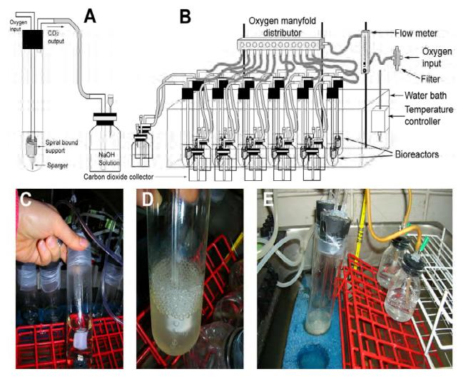
Figure 1. Minibioreactor experimental set. Diagram of minibioreactor of bubble column type showing connection to CO<sub>2</sub> collector vial (A). Diagram of a battery of minibioreactors (B). Close-up photographs of minibioreactors (C-E).
