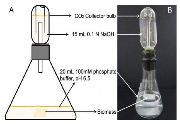
Figure 2. Diagram (A) and photograph (B) of the device used for measuring endogenous respiration.
