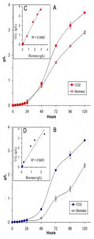
**Figure 4.** Biomass and carbon dioxide evolution kinetics of *Aspergillus niger* biofilm (A) and submerged (B) fermentations. Inserts show correlations between carbon dioxide evolution and biomass in biofilm (C) and submerged (B) fermentations. Error bars on the graph represent four replicates.
