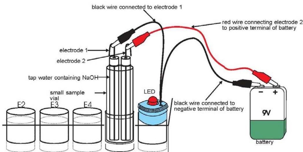
Figure 9 Electrolysis of water – microscale set-up
