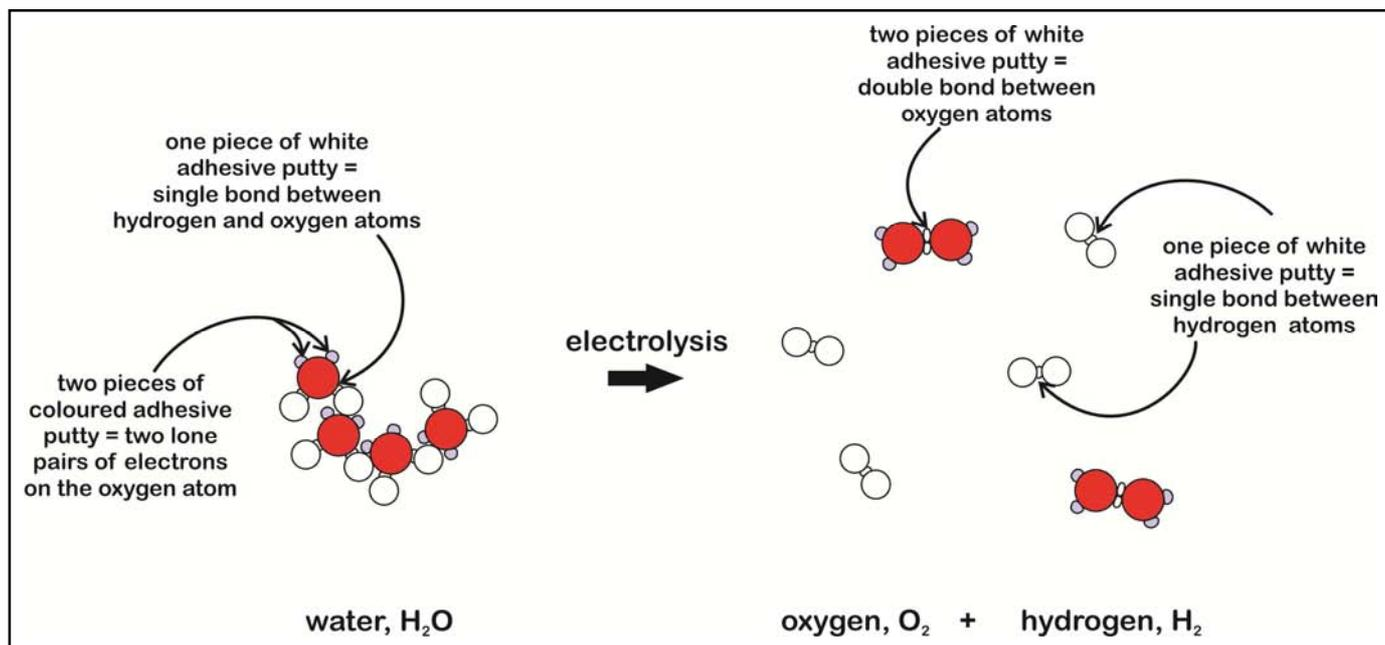
Figure 11 Electrolysis of water – 3-D modeling
