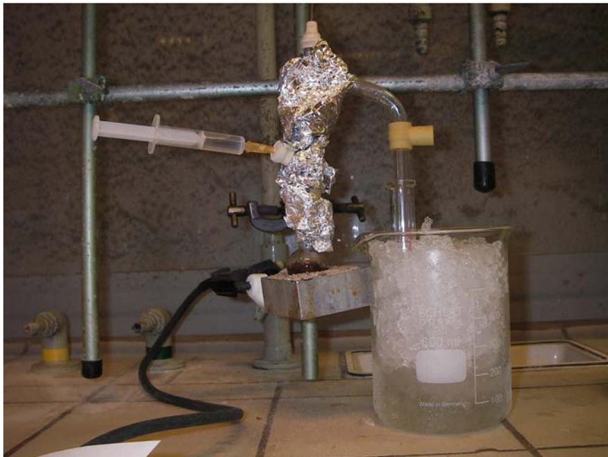
Figure 10. An example of an experimental setup for steamdistillation made by students using the Kontes set
