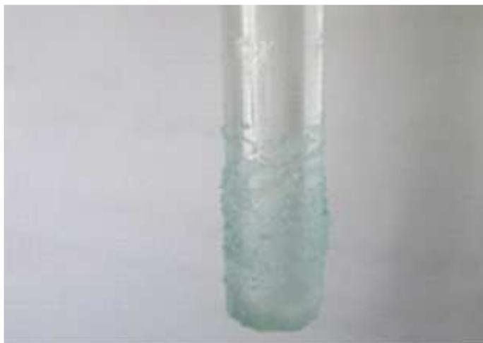
Figure 3 A photograph of APS-modified silica sensor after 30-minute exposure to the 500 ppm  $\text{Cu}^{2+}$  solution
