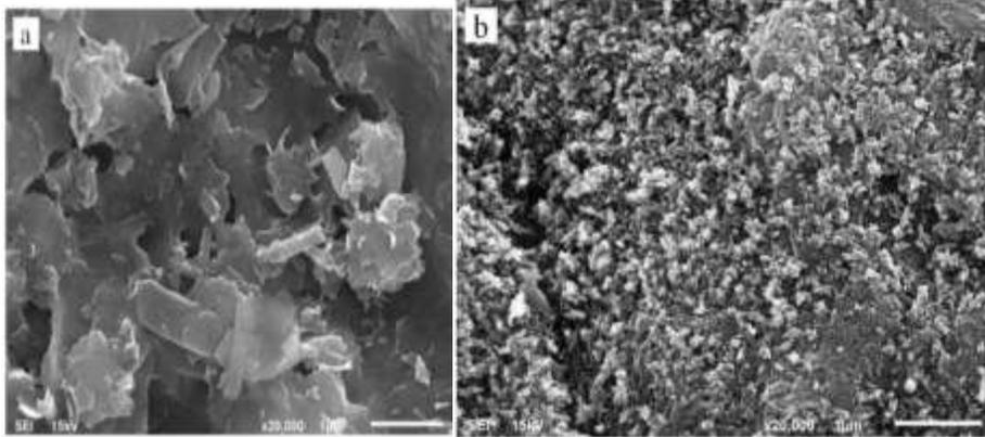
Fig (5) SEM image of a. Natural Bentonite and b. TiO<sub>2</sub>/ Bentonite composite [16].
