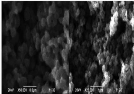
Fig (4) (a) SEM OF TiO<sub>2</sub> [15].
