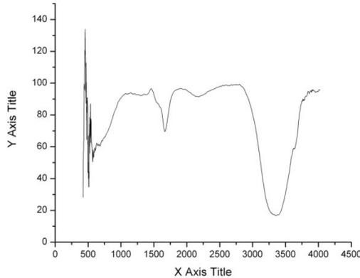
Fig (2): FTIR pattern of Chitosan. [14]
