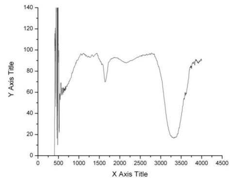
Fig (3): FTIR pattern of Chitosan/TiO<sub>2</sub> nanocomposites. [14]
