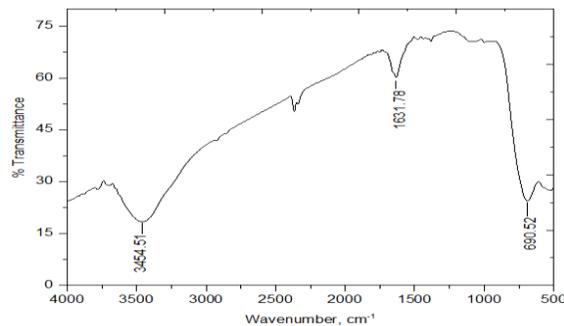
Fig (1): FTIR- Spectrum of TiO<sub>2</sub> [14].
