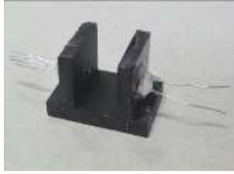
(Fig. 11) U-shaped acrylic stand with RGB LED and LDR CdS photoresistor
