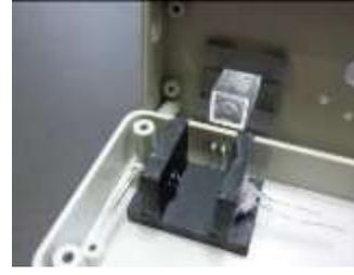
(Fig. 12) Cavity compartment allowing cuvette to go through
