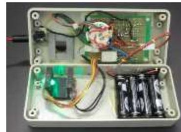
(Fig.15) Wired PC board, detached upper and lower parts of the plastic case
