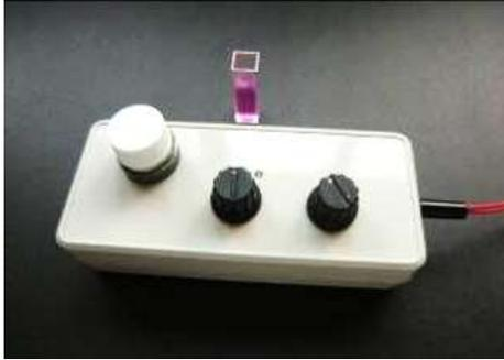
(Fig. 1) Full set of colorimeter sensor
