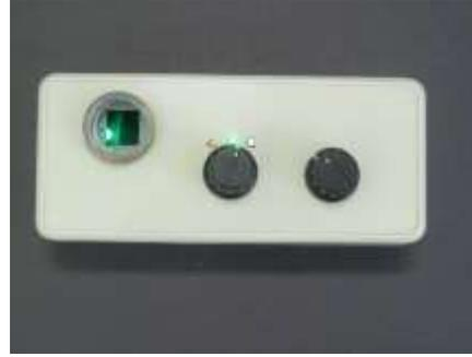
(Fig. 2) RGB tri-colour light source and cuvette compartment
