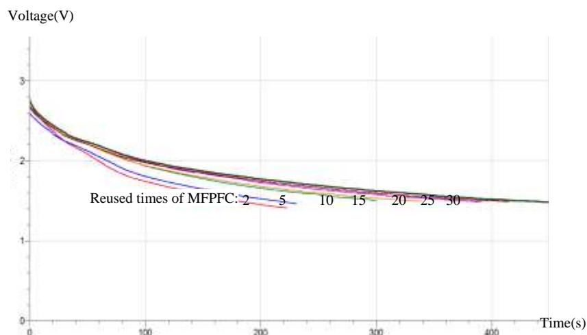
(Fig. 8) Voltage decay displayed by the used repeatedly MFPPC
