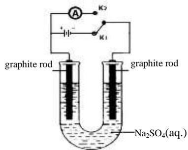
(Fig. 1) Traditional experiment of oxygen-hydrogen fuel cell in textbook
