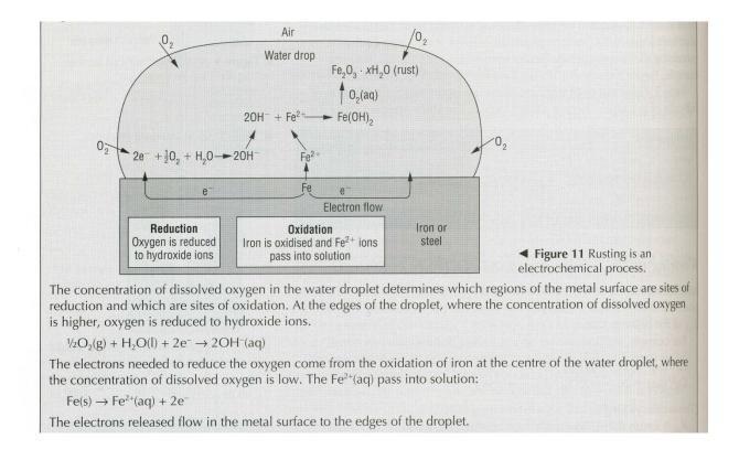
**Fig. 6:** Model drawing of most involved particles in the formation of rust (2)
