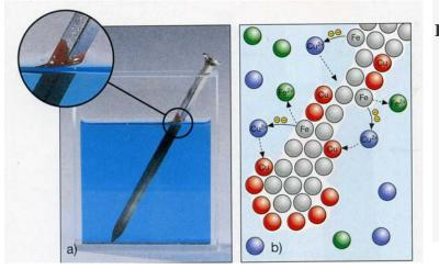
**Fig. 2:** Photo of the reaction of an iron nail with copper sulfate solution, model drawing of the particle view (1)
