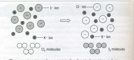
**Fig. 3:** Model drawing of the reaction of  $Cl_2$ molecules with I<sup>-</sup>(aq) ions, K<sup>+</sup>(aq) ions remain as spectator ions (2)
