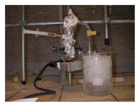
Figure 10. An example of an experimental setup for steamdestillation made by students using the Kontes set
