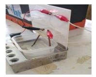
Figure 2. Small-scale setup (MyLab) for electrical conductivity test of ionic solutions
