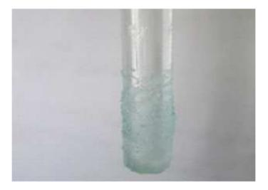
Figure 3 A photograph of APS-modified silica sensor after 30-minute exposure to the 500 ppm Cu2+ solution
