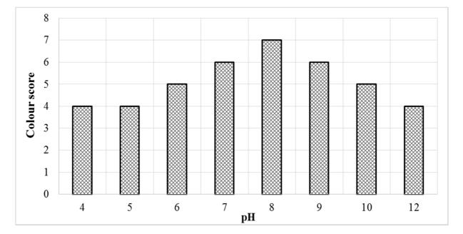
Figure 6 The effect of pH of the test solution on the effectiveness of the sensor (score /10)
