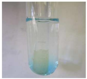
Figure 5 A photograph of glycine-modified APS-silica probe suspended in 500 ppm copper solution
