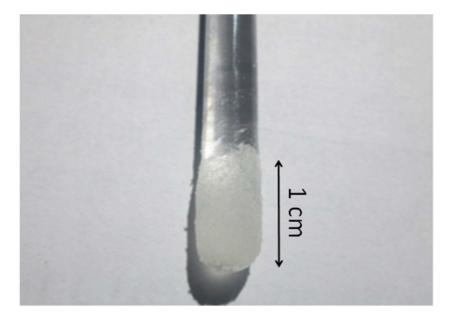
Figure 1 A photograph of the sensor: silica powder coated on the glass rod
