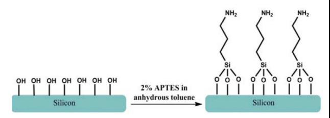
Figure 2 Schematic of presentation of APS modification of silica
