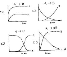
surplus or deficit concentrations of reactants and/or products [6, 7]. This is particularly true with respect to non 1:1 stoichiometric reactions. Typical student generated curves are shown in Figure 2. Frequently, the rendered plots have amounts of concentration spontaneously and incorrectly appear or disappear (Top and bottom left).
