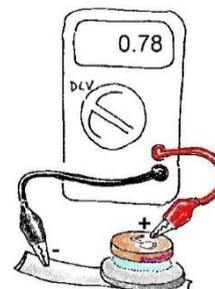
Add another strip of aluminium to the top and hold it down with an extra coin. Connect it to the other spring.
