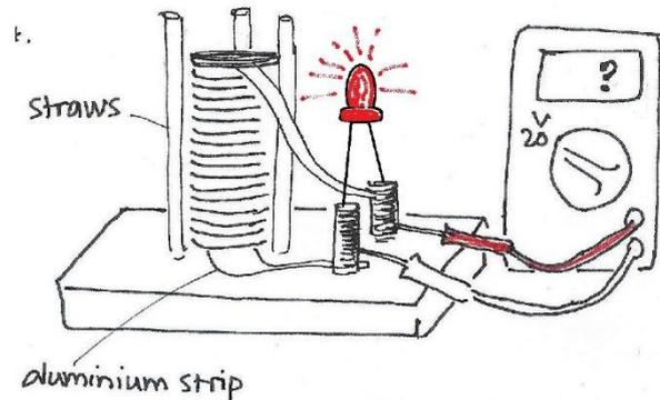
A red LED will glow when the p.d. across it is about 1.8 volts, and the current is about 0.02 ampere.
