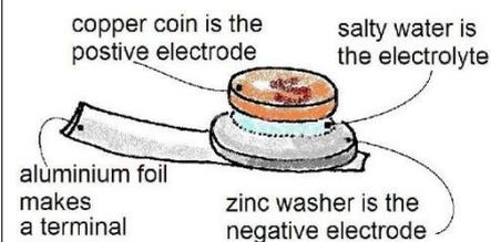
**Figure 3** Measure the p.d. between the zinc and the copper.
