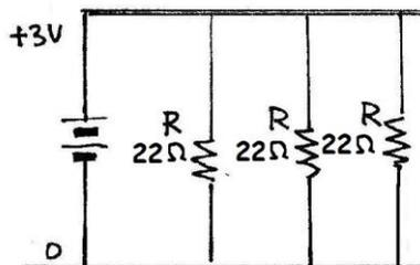
You don't have 1 ohm resistors so use the 22 ohm resistors instead.
