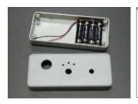
(Fig. 7) Upper (with holes) and lower (with battery holder) parts of plastic case (Fig. 8) Medicine bottle, cap and cuvette adapter
