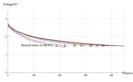
(Fig. 8) Voltage decay displayed by the used repeatedly MFPFC
