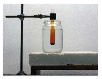
Figure 1: Experimental setup for the reaction of aluminum and bromine
