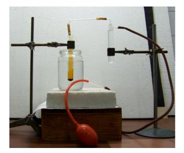
Figure 2: Adding water to the reaction product using the safety dropper.
