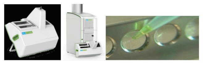
**Figure 2.** From left to right, direct sampling port, Time of Flight piece of the instrument TOF-MS and picture of sample application on to the disposable wire mash.
