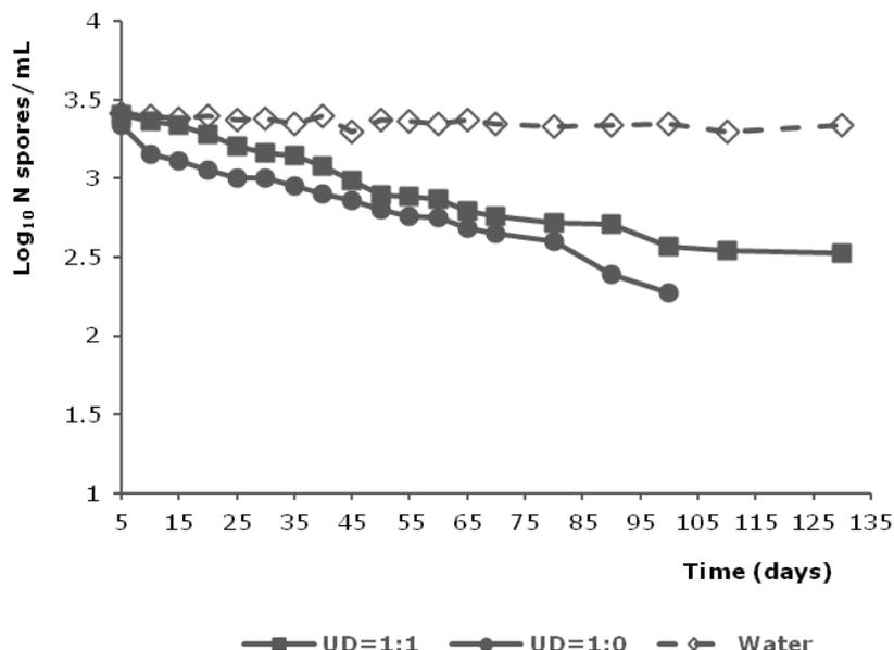
**Figure 2.** Reduction of *C. perfringens* spores during samples exposure at ambient temperatures. The initial values were 8260 mg/L NH<sub>4</sub>-N (pH 8.8) for the undiluted urine (●); 4450 mg/L NH<sub>4</sub>-N (pH 8.7) for the half-diluted urine (■) and pH 7.4 for the control (◇).
