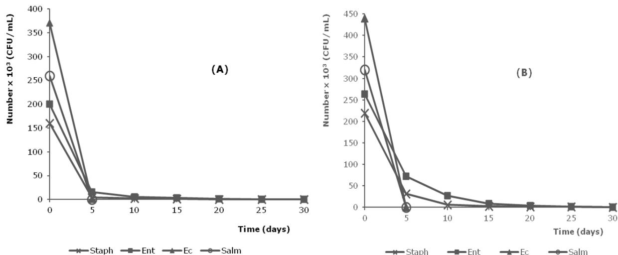
**Figure 1.** Reduction of bacterial numbers (*E. coli* [▲], *Salmonella* sp. [○], *S. aureus* [X], *E. faecalis* [■]) during samples exposure at ambient temperatures. The initial values were 8260 mg/L  $\text{NH}_4\text{-N}$  (pH 8.8) for the undiluted urine (A) and 4450 mg/L (pH 8.7) for the half-diluted urine (B).
