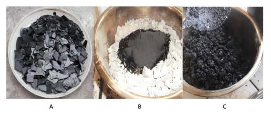
**Figure 8.** The plastic bags powder used alone as binder for concretes: platelets of the melted waste plastic bags (A), melting of powder on aggregates (B) and decoulant concrete ready to be molded (C).
