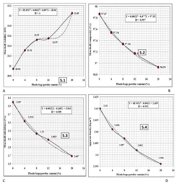
**Figure 5.** Effects of the added molten plastic bags powder contents on Marshall' stability (A), Subsidence (B), Compacity (C) and Apparent density (D) of doped bituminous concretes (solid lines = experimental data curves; dash lines = trend curves).
