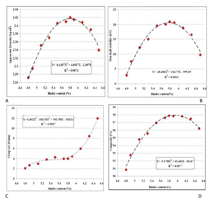
**Figures 4.** Evolutions of Apparent density (A), Marshall' stability (B), Creep (C) and Compacity (D) of the tested bituminous concretes as function of percentage of control 50/70 graded bitumen (M<sub>0</sub>).
