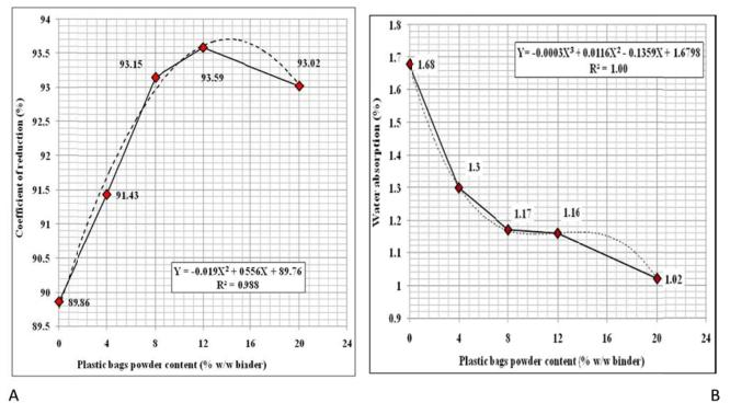
**Figure 7.** Duriez testing results: respective behaviors for water absorption rate at (1-day in controlled air + 7-days water immersed at 18 °C) (A) and reduction coefficient (B) of bituminous concretes versus plastic bags powder content.
