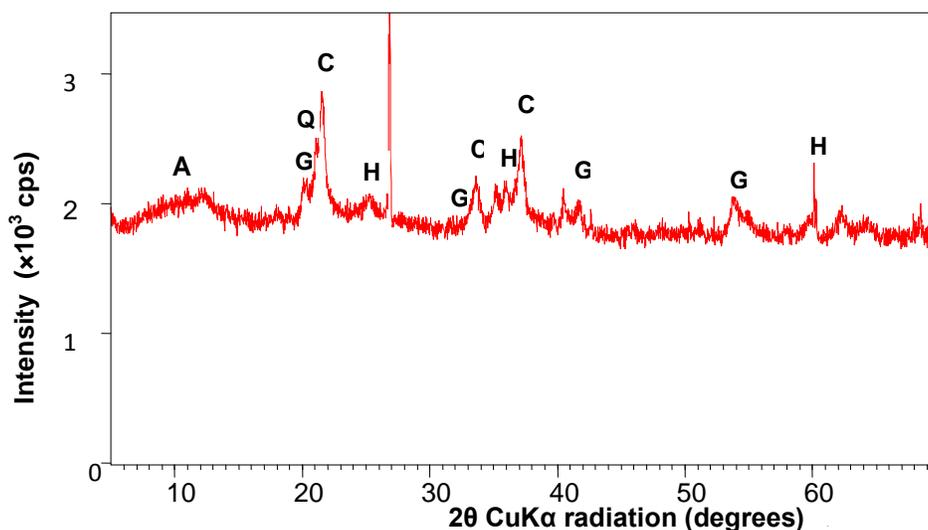
**Figure 1.** XRD pattern of Lateritic mineral adsorbent material (LM-1), Q=Quartz, C=Cristobalite, G= Goethite, H = Haematite, A = Contribution from Amorphous matrix.
