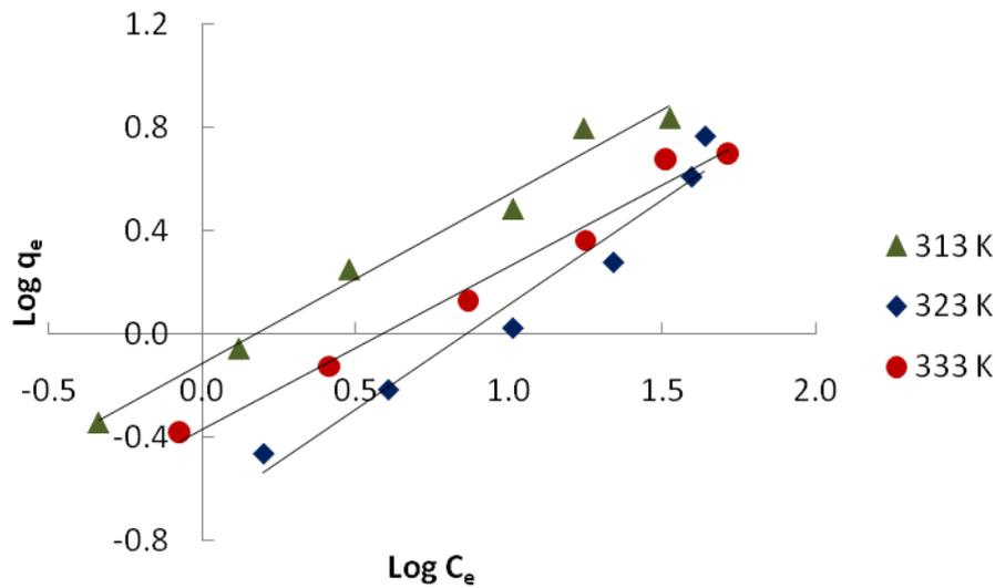
**Figures 9.** Freundlich adsorption isotherms for F adsorption onto LM-1 at 313 K, 323 K and 333 K.
