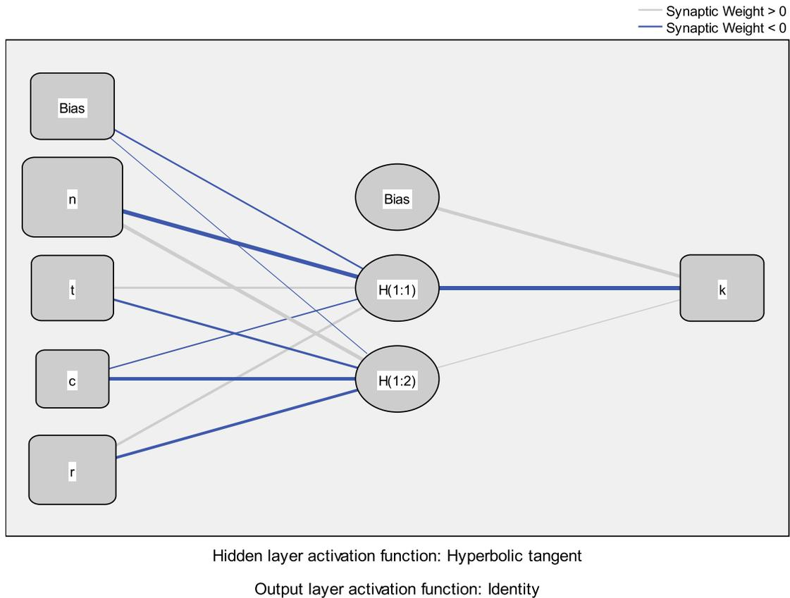
**Figure 2.** Network diagram. n-represents the sunshine hour; t-represents maximum temperature; c-represents cloud cover; r-represents relative humidity and the output k-represents clearness index.
