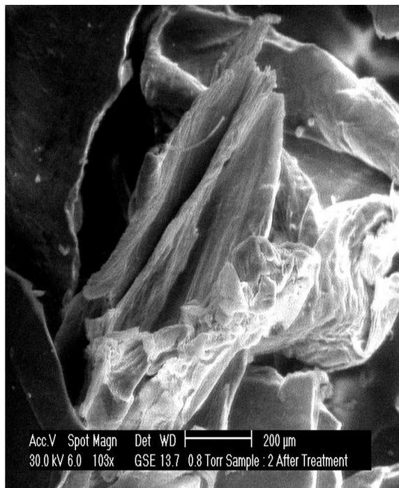
**Figure 3.** SEM analysis of chitin after adsorption of dye.
