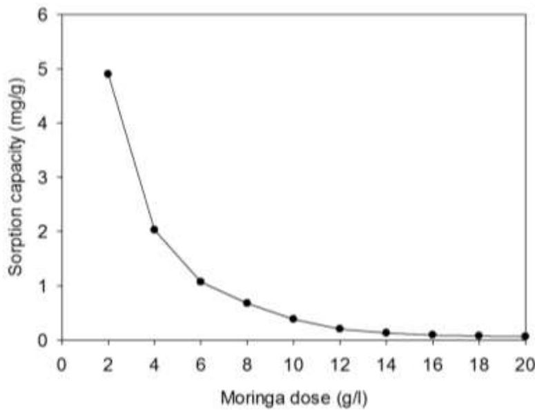
**Figure 4.** Sorption of capacity of Fluoride ion at different dosage of *Moringa*, initial concentration 10 mg.L<sup>-1</sup>, pH ±7, volume of test solution 250 ml, contact time 60 min.
