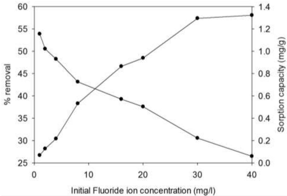
**Figure 3.** Effects of initial Fluoride ion concentration on biosorption by *M. stenopetala*, initial fluoride ion concentration 0 to 40 mg. L<sup>-1</sup>, *Moringa* dosage 2 g, volume of test solution 250 ml, pH ±7, contact time 60 min.
