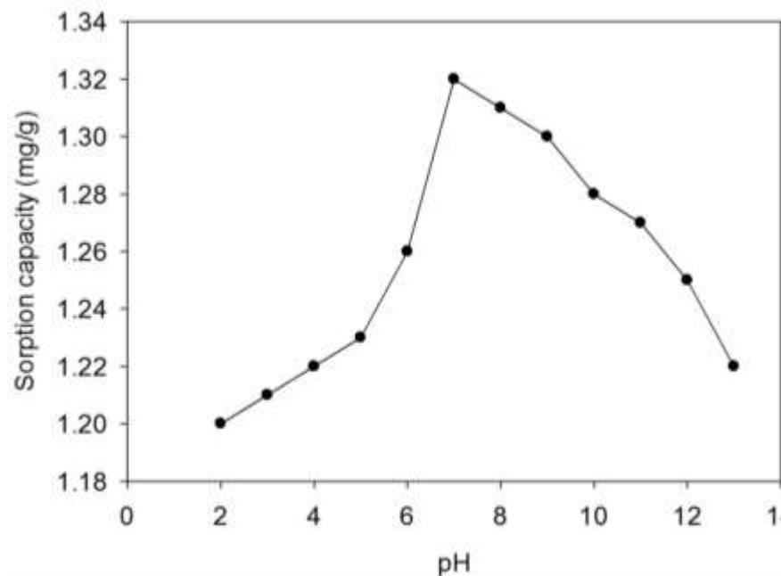
**Figure 2.** Effects of pH on fluoride ion sorption capacity of *M. stenopetala* seeds , initial fluoride ion concentration of  $10 \text{ mg.L}^{-1}$ , *Moringa* dosage 2 g, volume of test solution 250 ml, contact time 60 min.
