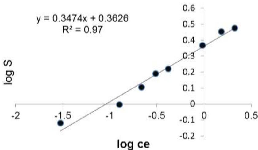
**Figure 6.** Freundlich isotherm for adsorption of Fluoride ion, initial Fluoride ion concentration 0 to 40 mg. L<sup>-1</sup>, *Moringa* dosage 2 g, volume of test solution 250 ml, pH ±7, contact time 60 min.
