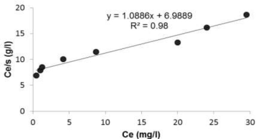
**Figure 7.** Langmuir Isotherm for adsorption of fluoride ion, initial Fluoride concentration 0 to 40 mg. L<sup>-1</sup>, *Moringa* dosage 2 g, pH ±7, volume of test solution 250 ml, contact time 60 min.
