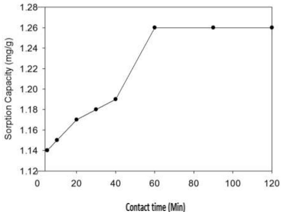
**Figure 1.** Sorption of Fluoride ion as a function of contact time initial  $F^-$  concentration of  $20 \text{ mg.L}^{-1}$ , *Moringa* dosage of 2 g, volume of test solution 250 ml, pH  $\pm 7$  and contact time 5 to 120 min.
