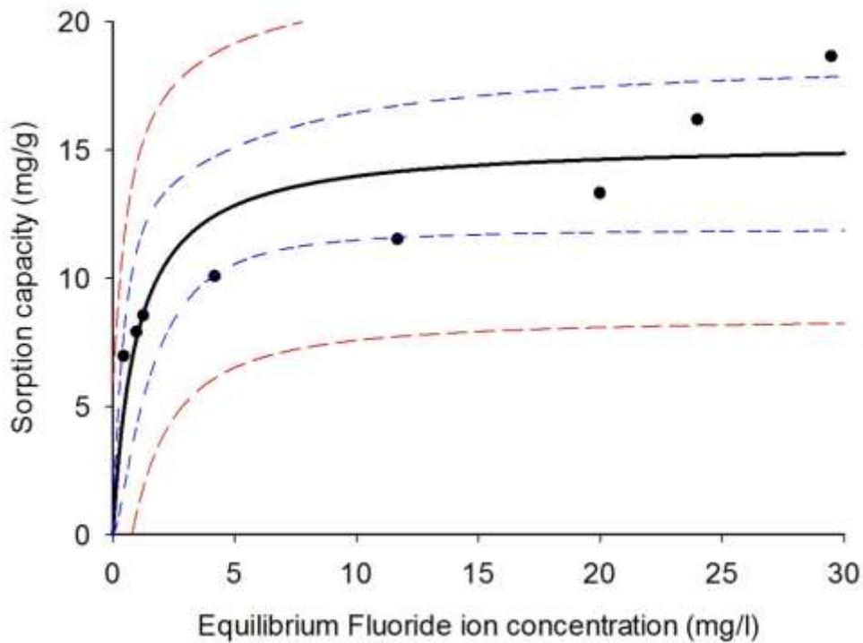
**Figure 8.** Binding of fluoride ion on *Moringa stenopetala* powder, initial fluoride ion concentration 0 to 40 mg. L<sup>-1</sup>, *Moringa* dosage 2 g, pH ±7, volume of test solution 250 ml, contact time 60 minutes. Solid line = Sorption capacity vs. Equilibrium fluoride ion concentration; black dots = Sorption capacity vs. Equilibrium fluoride ion concentration; Short-Short line = 95% confidence band; Medium dash line = 95% prediction band.
