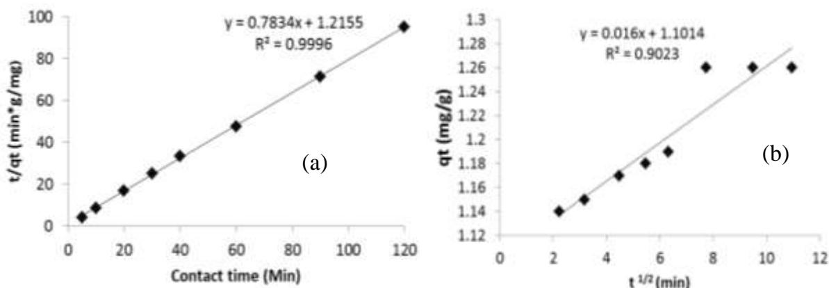
**Figure 5.** Plot of pseudo-second-order model (a) and Intraparticle diffusion model (b) for fluoride ion adsorption onto *Moringa* powder. Initial Fluoride ion concentration 20 mg. L<sup>-1</sup>, *Moringa* dosage 2 g, volume of test solution 250 ml, pH ±7.
