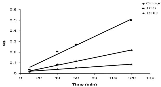
Figure 5. Pseudo second order plot for adsorption of colour, BOD and TSS using boiler fly.
