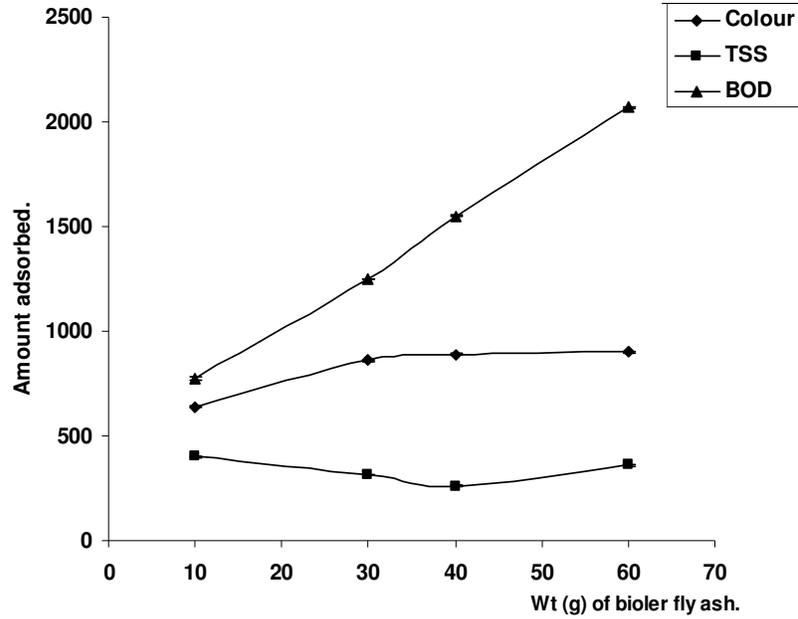
**Figure 1.** Amount adsorbed against weight of boiler fly ash for adsorption of colour (Hz), TSS (mg/g) and BOD (mg/g) from palm oil mill effluent using boiler fly ash of particle size 425 µm.
