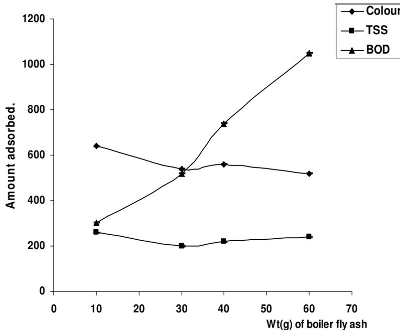
**Figure 2.** Amount adsorbed against weight of boiler fly ash for adsorption of colour (Hz), TSS (mg/g), and BOD (mg/g) from palm oil mill effluent using boiler fly ash of particle size 850µm.
