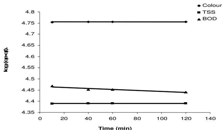
**Figure 4.** Pseudo first order plot for adsorption of colour, BOD and TSS using boiler fly ash.
