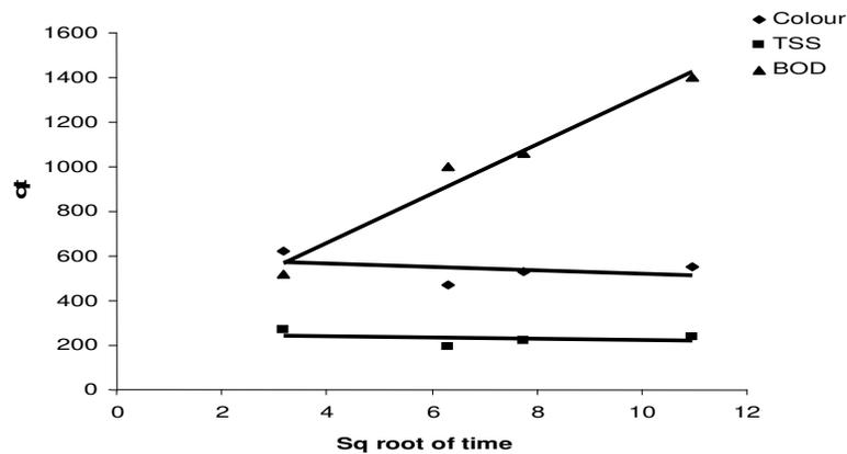
Figure 6. Intraparticle diffusivity plot for adsorption of colour, BOD and TSS using boiler fly ash.
