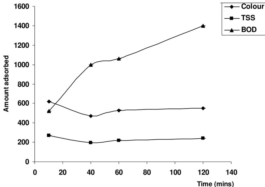
**Figure 3.** Amount adsorbed against time (mins) for adsorption of colour, TSS and BOD from palm oil mill effluent using boiler fly ash.
