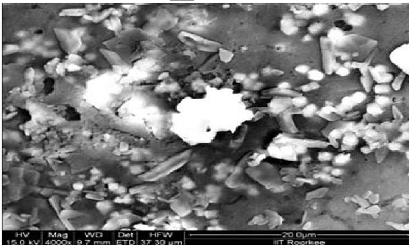
**Figure 2.** Scanning electron micrograph of tea waste biomass.
