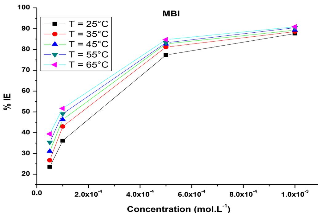
Figure 5. Variation of Inhibition efficiency with inhibitor (MBI) concentration at different temperatures.
