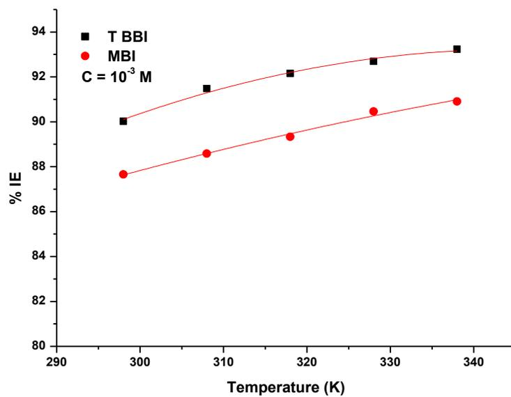
Figure 8. Inhibition efficiency of the studied inhibitors (TBBI and MBI) as a function of temperature.
