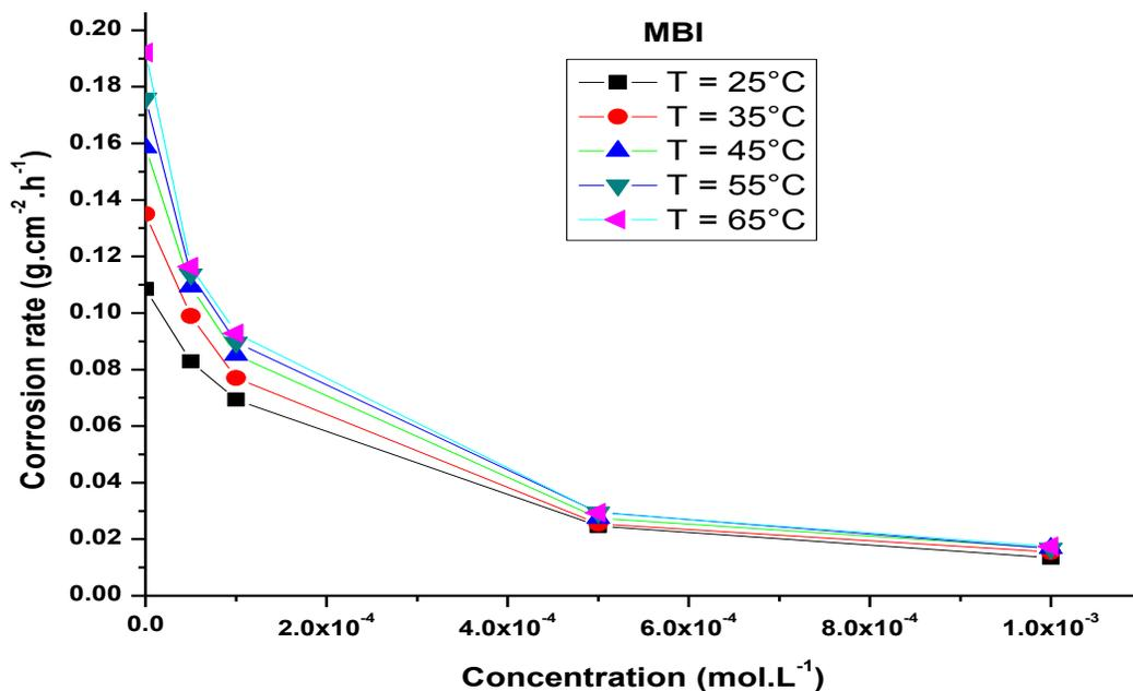
Figure 3. Variation of corrosion rate with inhibitor (MBI) concentration at different temperatures.
