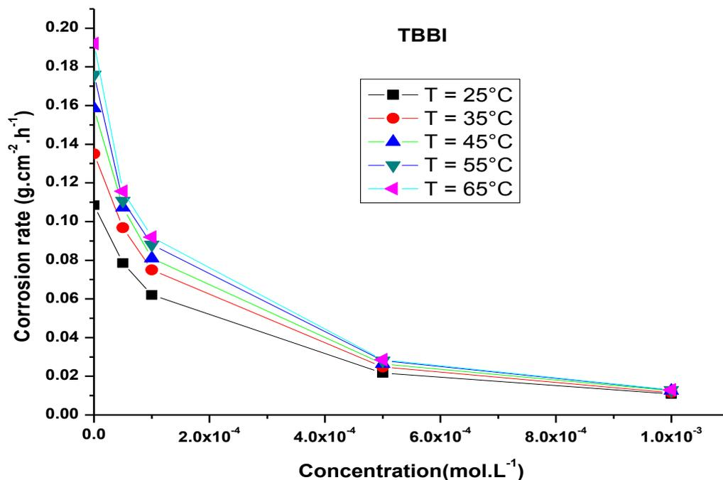
Figure 2. Variation of corrosion rate with inhibitor (TBBI) concentration at different temperatures.
