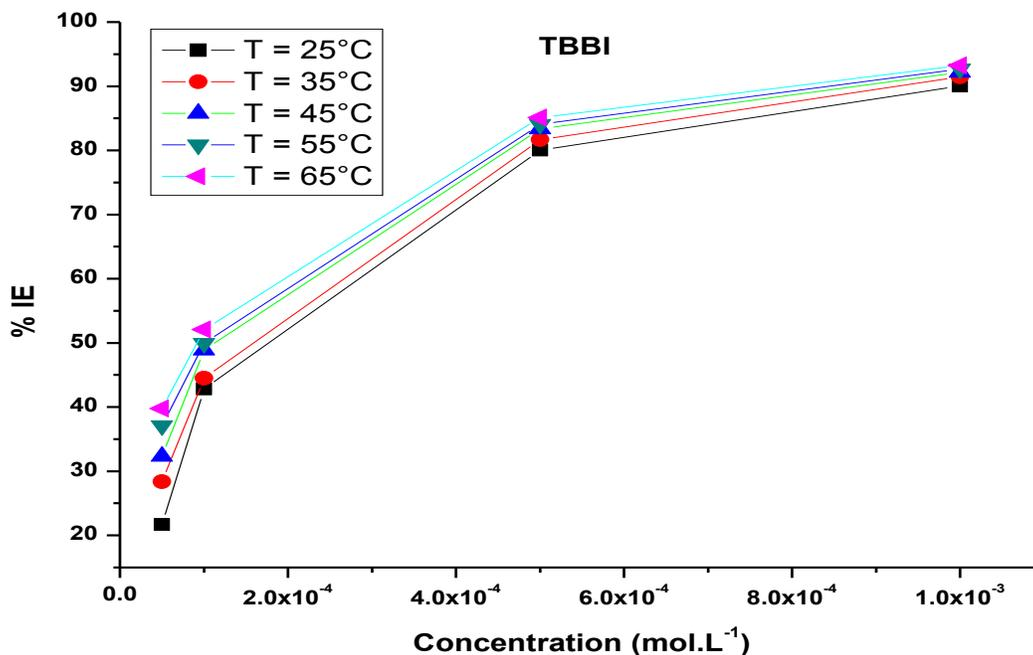
Figure 4. Variation of Inhibition efficiency with inhibitor (TBBI) concentration at different temperatures.
