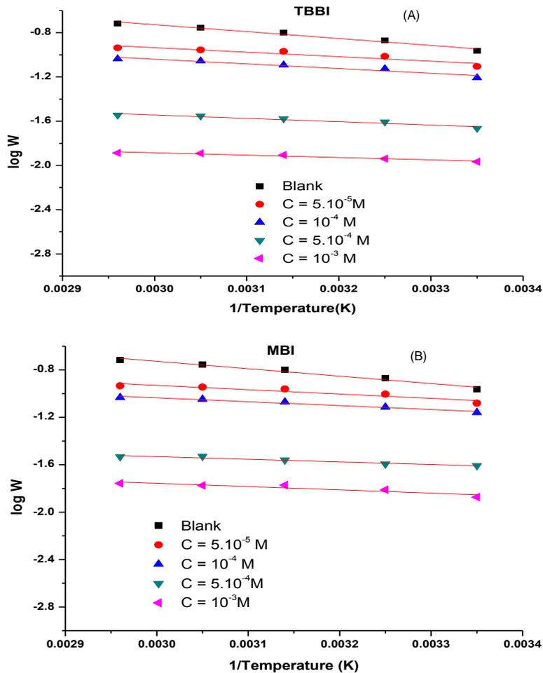
Figure 7. Arrhenius plots for copper corrosion in 1M HNO<sub>3</sub> without and with different inhibitor concentrations (a): TBBI (b): MBI.
