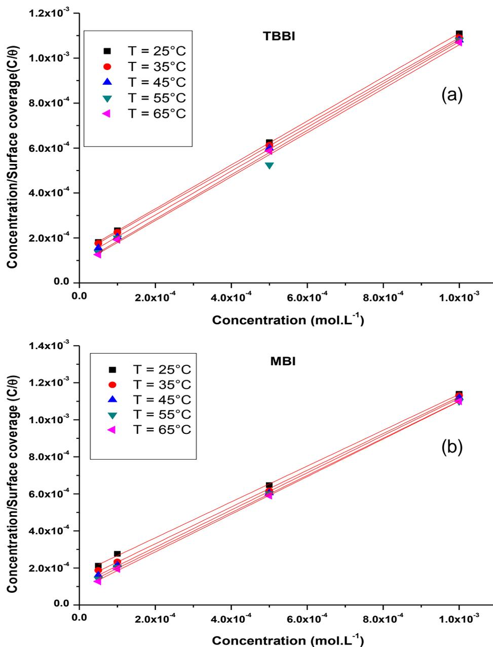
**Figure 6.** Langmuir adsorption plots for copper in 1 M HNO<sub>3</sub> containing various concentrations of inhibitor at different temperatures. (a) TBBI (b) MBI.
