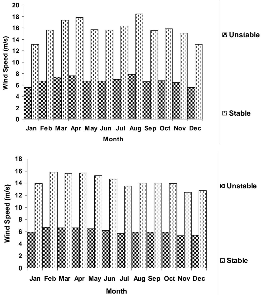
**Figure 1.** Variation of calculated mean monthly wind speeds in Lagos (upper panel) and Calabar (lower panel) using power law relationship.
