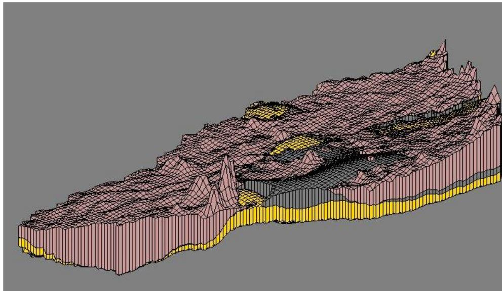
Figure 6. 3D image of the lithology of the study area created by using GMS visualization tools.
