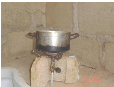
Figure 3. Cooker burner using biogas.
