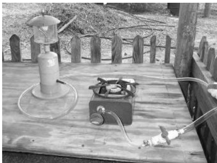
Figure 9. Modified gas stove and pressure lamp attached to biogas storage container. Source: Forst (2002).
