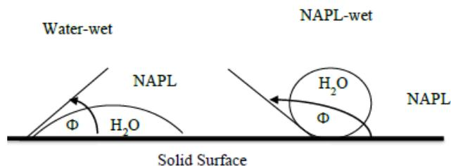
**Figure 1.** Contact angle, wetting and non-wetting interface (Mercer, 1990).
