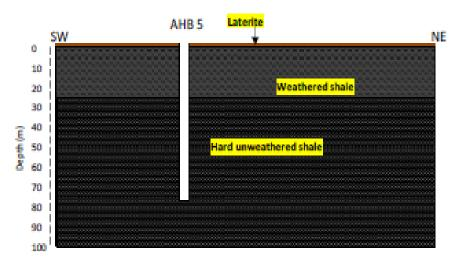
Figure 11. Schematic sections from the surveyed area (VES 5).
