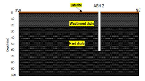
Figure 8. Schematic sections from the surveyed area (VES 2).
