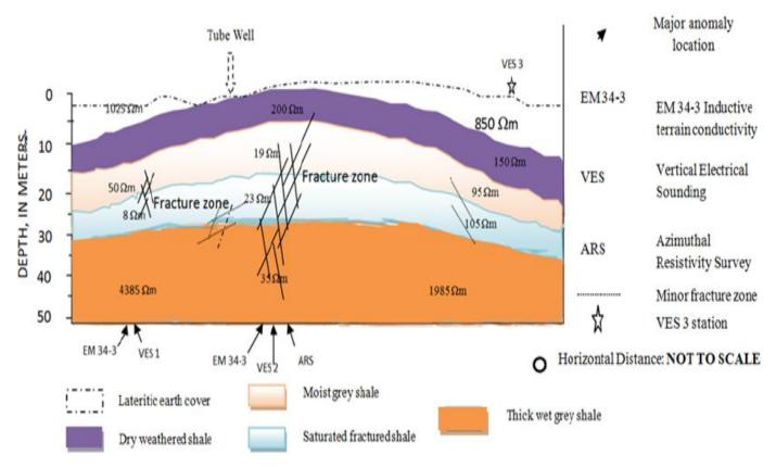
Figure 12. The distribution of fracture zones in the Kpiri Kpiri area of Abakaliki, southeastern Nigeria (Odoh et al., 2012).
